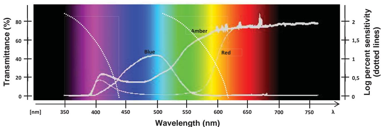
**Figure 4.** Transmission spectrum of the blue, red and amber igloos (solid lines) and the relative sensitivity of the known photopigments of the murine eye. UV cone with a  $\lambda_{\text{max}}$  at 359 nm and M cone with a  $\lambda_{\text{max}}$  at 509 nm (broken lines).
