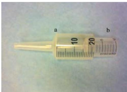
**Figure 1.** Syringe B is inserted into syringe A. a: A 50 ml syringe, b: A 20 ml syringe.
