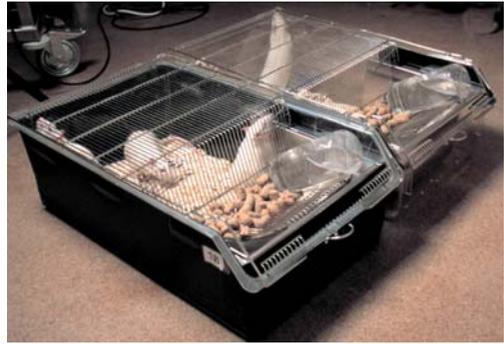
**Figure 2.** Illustration of cages with polycarbonate body and inner stainless steel half cage (Oulu), one of the cages has a non-transparent plastic covering.
