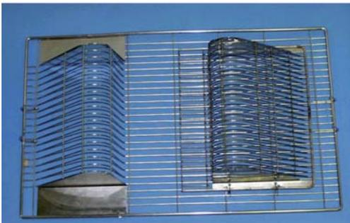
**Figure 1.** Illustration of cages with stainless steel body and polycarbonate inner half (Kuopio). In the left side cage, there is a cover with a false food hopper. The figure below shows the structure of the cover with the original and a false food hopper.
