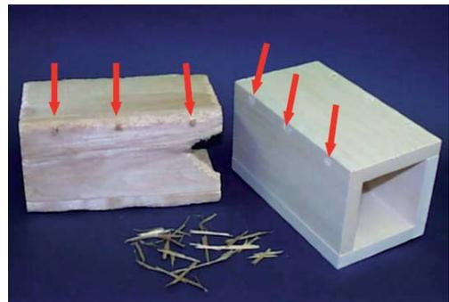
**Figure 1.** Picture of new (right) and partly gnawed used tube (left). Fragment of aspen wood from other tubes appear at the front of the tubes. The three pins joining the boards at each corner are shown with the red arrows.
