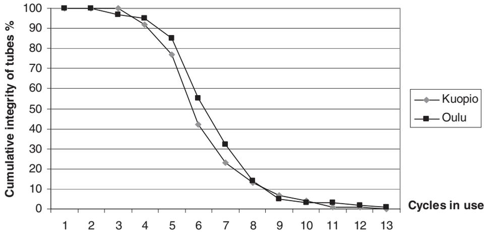
**Figure 2.** Cumulative mean disintegration of aspen tubes (n = 120) after each cycle (= 0.5 weeks). The tubes were autoclaved before use and after each cycle in use.
