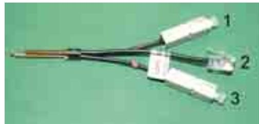
**Figure 1.** Probe made entirely of PSU for the measurement of intramedullary perfusion and temperature near the cortex, with integrated afferent and efferent optical fibre cables and cable for the temperature sensor, and the jacks for connection with the laser Doppler and temperature measurement units. 1: Efferent optical fibre cable, jack. 2: Cable for temperature measurement, jack. 3: Afferent optical fibre cable, jack.
