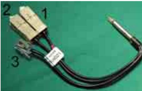
**Figure 3.** Probe for the measurement of intramedullary perfusion and temperature near the bone cortex, with metal reinforcement in the rear area and the jacks for connection with the laser Doppler and temperature units. 1: Afferent optical fibre cable, jack. 2: Efferent optical fibre cable, jack. 3: Cable for temperature measurement, jack.
